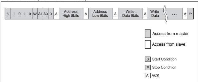
Note: It is not necessary to take a period for internal write operation cycles from the buffer to the memory after the stop condition is generated.
